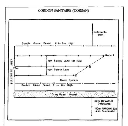
Mine laying was carried out in patterns according to ropes marked with notes. Three ropes, each 50 metres long, were laid parallel to each other. These rows are ten yards apart within the 25 metre-wide strip. Ropes were designated 'rope A, B, and C'. Rope 'A' was knotted at 1 metre intervals while 'B' was at every 2 metres and 'C' at every 3 metres.
